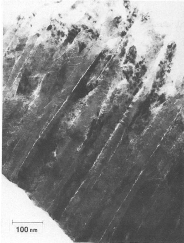
Figure 3 Bright field transverse micrograph of film B [NN8535] showing NbN columnar grain in the middle portion of the film.
